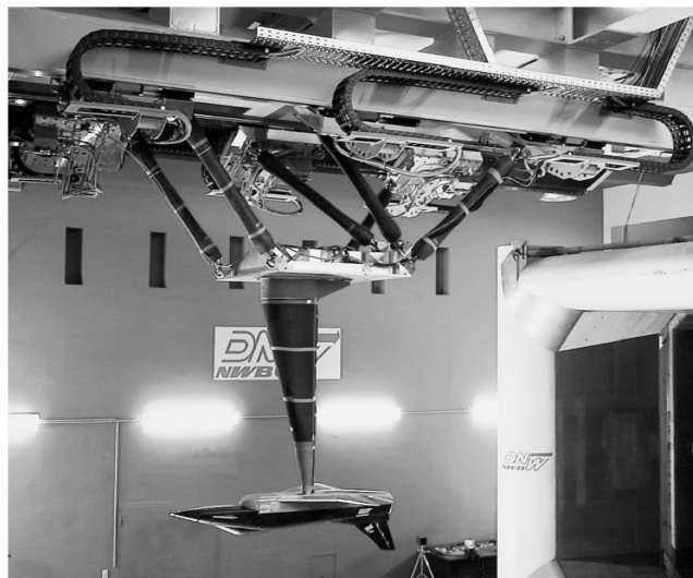
Fig. 1 Model positioning mechanism (MPM) with belly sting and X-31 remote-control model in the low-speed wind tunnel NWB.
